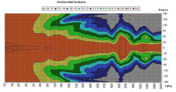
Parameters: Cyclic Move: 0°; Symmetry: average sym; Freq.Smooth; 1/3 Oct; Ang.Resol.: 5°; Rel. to: 0° Axis 0°
